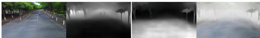
Fig. 6. Images without improvement. Clear image; Depth map; Transmission map; Fog simulation image
