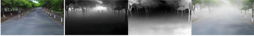
Fig. 7. Images with improvement. Clear image; Depth map; Transmission map; Fog simulation image
