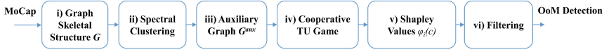
Fig. 1. Main steps of the algorithm developed by Kolykhalova et al. [19] for the automated detection of the perceived OoM.
