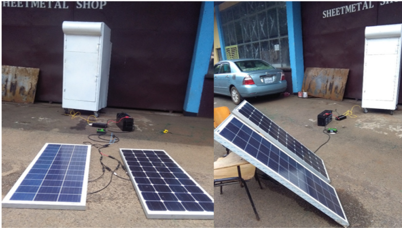
Fig. 3. Pictures of experimental test set up of evaporative cooling
