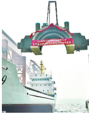
Fig. 1. First AP1000 nuclear power turbo-generator in the world
