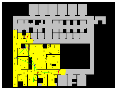
Fig. 6. Exploration snapshot. Blue and red - not ready and ready UAVs. Green squares - The BS. Green lines - current communication links. (Color figure online)
