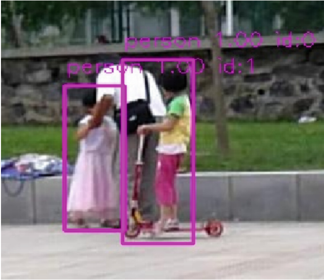
Fig. 9. The ID number displacement phenomenon occurs when the hidden dangers of the same type overlap with each other (Frame 54 comes with a normal ID number)
