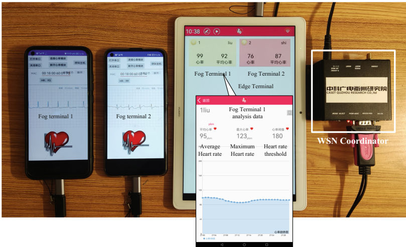
Fig. 7. Edge terminal and sample heart rate data
