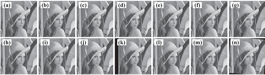
Fig. 7. Watermarked image “Lena” suffered different attacks, and a–n represent GN (0.02%), SN (0.1%), SPN (1%), AF (3×3), WF (3×3), GLPF (3×3), MF (3×3), JPEG (QF = 70), RE (0.5), RE (2), CR (10%), MB (4, 7), SH (0.8), RO (5°), respectively.
