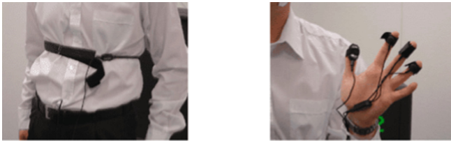
Fig. 2. Respiration sensor and Skin conductivity, temperature and Finger blood volume pulse (BVP) sensor [1, 6].
