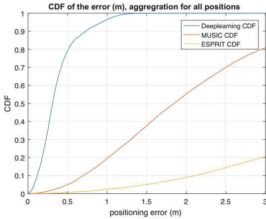
Fig. 6. Comparison of cumulative distribution function of positioning error in outdoor LOS test.
