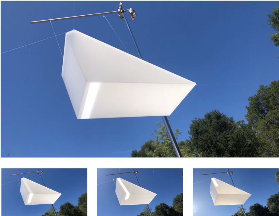
Fig. 6. Photos demonstrate the design prototype using Lighting White 60% plexiglass. The top image shows light entering into the structure precisely at midday near to June solstice. The following three photos show the light as it enters into the structure after midday. Photos taken by Emma Strebel.
