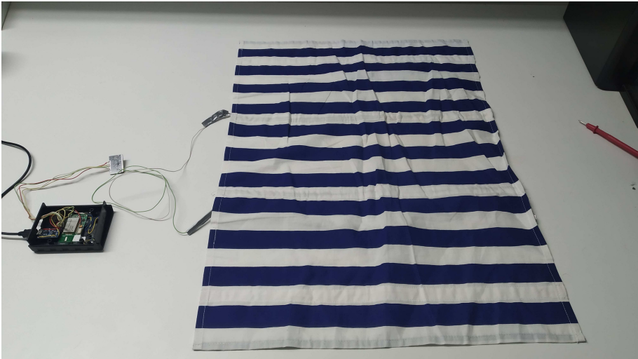
Fig. 7. Photo of the actual bed activity sensor implemented, using only “of the shelf” IoT components.
