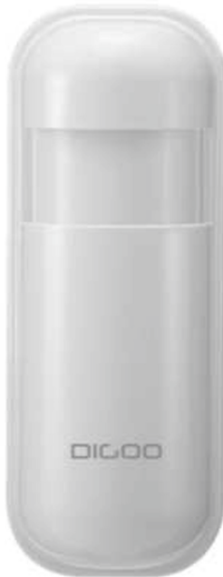
Fig. 5. Picture of the actual PIR activity sensor implemented, using only “of the shelf” IoT components.
