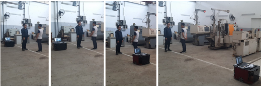
Fig. 13. Data fusion between 2D lidar and digital camera for human detection [58].
