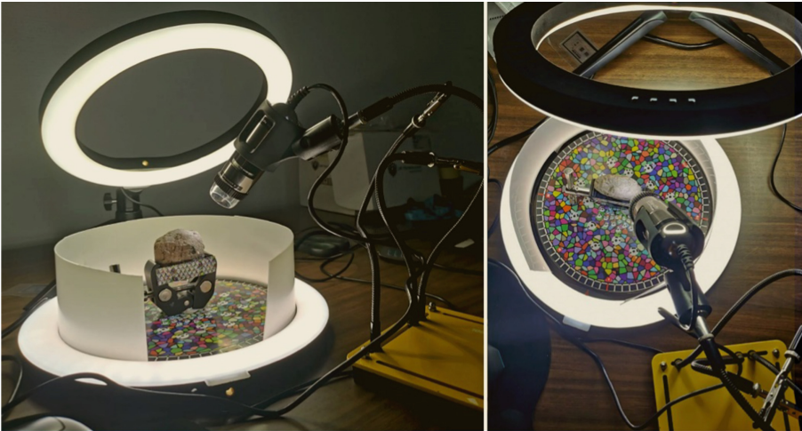
Fig. 2. A turntable- and clamp-based acquisition system with ring illumination that supports integrated LED lighting for the microscope. The USB microscope is fixed on a plastic microphone holder customized to be set to a plate with several flexible hooks.
