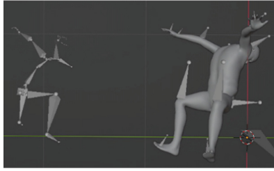
Fig. 6. A sample of common error in SMPL hip movements (right) versus MoCap (left).
