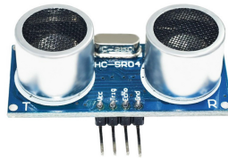
Fig. 4. Physical image of the HC-SR04 ultrasonic module.
