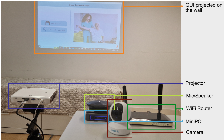
Fig. 5. All the hardware components used in the deployment of the proof-of-concept developed.
