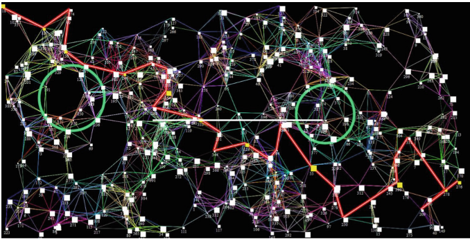
Fig. 3. Flight Path of UAV for 400 Data-points (Red line is flight path), White nodes: task points, yellow nodes: waypoints, Green circles: No Fly Zones (Color figure online)
