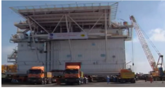
Fig. 1. The use of high-powered tractors to push or pull convoys of cargo trailers
