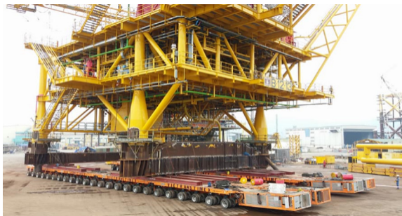
Fig. 2. A modern self-propelled trailers transporting oil-shore
