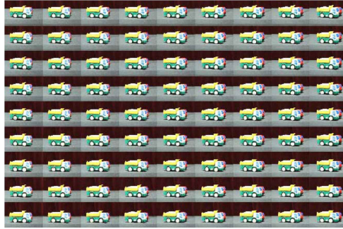
Fig. 4. Two dimensional multi view image array actually collected
