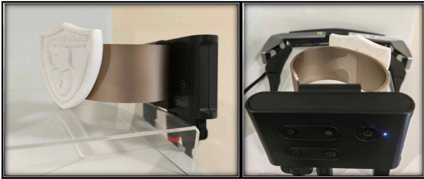
Fig. 7. A 3D printed bracelet connected to a virtual reality system Epson MOVERIO Augmented Reality Smart Glasses.
