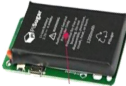
Fig. 13. Pi sugar battery for raspberry pi [21].
