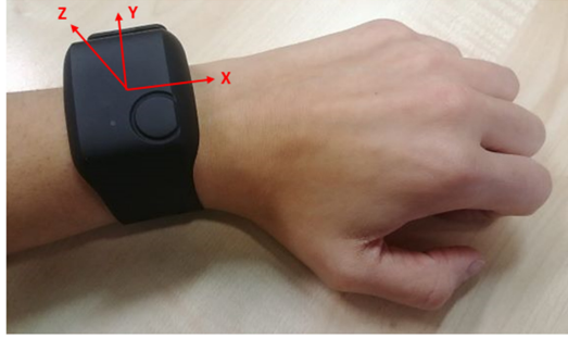
Fig. 1. Position of the wrist-worn Empatica E4 with the system of coordinates on the device.
