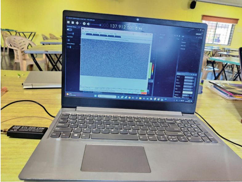
Fig. 2. Result of NOAA-15 (National Oceanic Atmospheric Administration) satellite which was tracked on 17th of June 2023. The process begins with capturing raw images from the NOAA-15 satellite. These images may contain various types of noise, such as electronic noise, and atmospheric interference.
