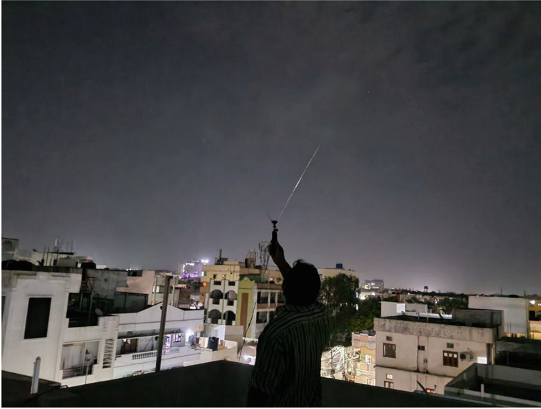
Fig. 3. V-dipole antenna is used to track the satellite. This antenna design is popular for satellite tracking due to its simplicity, omnidirectional properties, and effectiveness in receiving signals from various directions.
