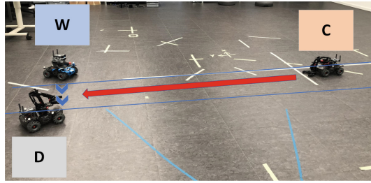
Fig. 2. Example of data collection scenario. Three RoboMasters devices are positioned on the laboratory floor where the dataset has been recorded. The device on the left acting as the wheelchair is labeled “W,” the one on the right representing the obstacle is labeled “C,” and the one at the bottom labeled “D” represents the drone. A red arrow runs horizontally from the left to the right show the trajectory of the obstacle. Blue chevrons pointing left near the bottom vehicle are equivalent to the pedestrian crossing. Blue lines run parallel to the red arrow, indicating the boundaries of the obstacle trajectory. (Color figure online)
