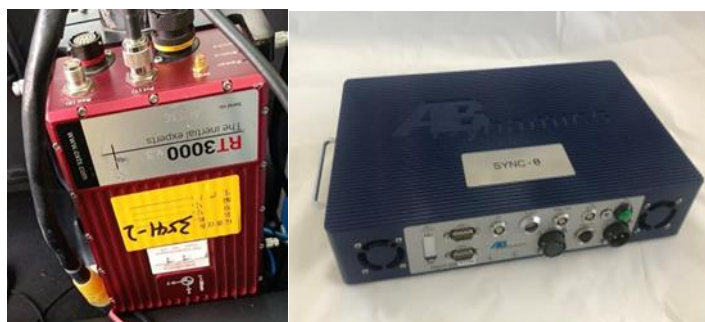
Figure 4. GPS Navigation Test System & Synchronization Controller
