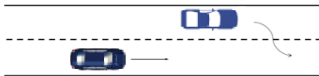
Figure 2. Schematic Diagram of Test Scenario for Cut-in
