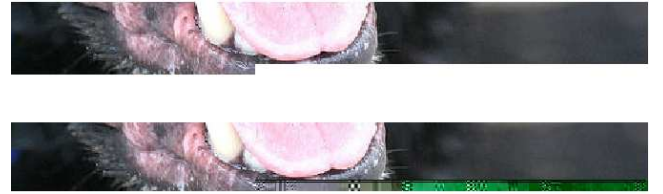
Figure 6: An example of an image corruption which can be revealed by decoding sectors one at the time. This image (of a dog) was taken from the 2007 DFRWS at header offset 87716 sectors. The top part is shown after decoding 243 sectors, while the bottom part was after decoding 244 sectors. The black bands illustrate the region over which the Estimate (Eq. 1) was taken. This region is restricted to the boundary between the smaller image and the image obtained by decoding more data.
