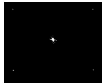
Fig. 5 : Fourier transform showing Bayer interpolation peaks.
