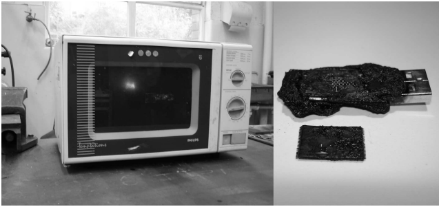
Figure 10: Left: a memory stick catches alight in a microwave oven. Right: the remains of the memory stick. The Flash memory die is visible through its damaged packaging.
