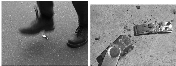
Figure 7: Left: A memory stick is stomped upon. Right: The remains of a memory stick after it has been struck 36 times with a hammer.
