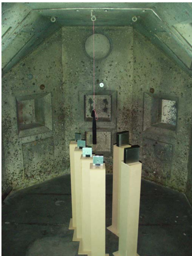
Figure 1. Four aluminium plates and two steel plates are located at the distances 0.25 – 1 m away from a 0.7 kg CompB charge.
