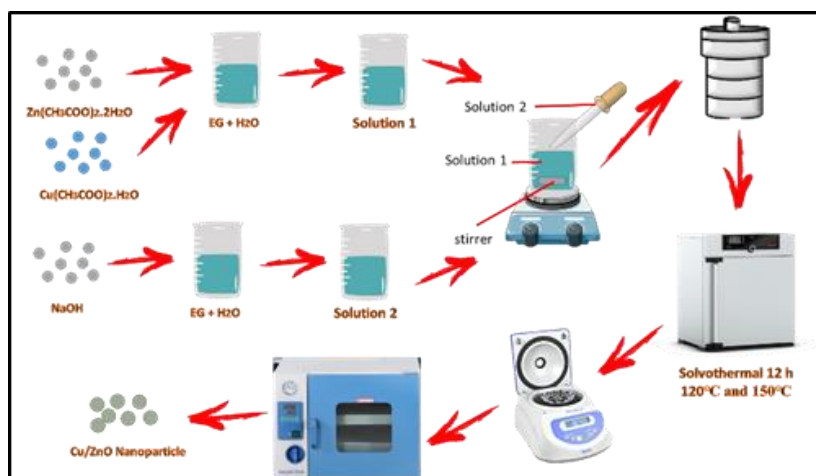
Fig. 9. Cu/ZnO Nanoparticle Synthesis Scheme with Solvothermal Method
