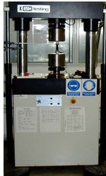
Figure 1. Sensor stressed by fatigue machine and connected to the Shimmer platform.
