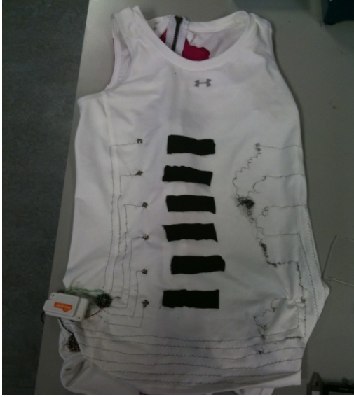
Figure 8. New shirt with 6 sensors connected to Shimmer platform.
