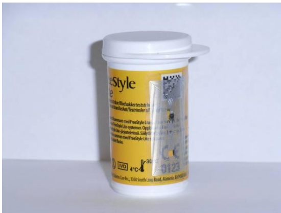
Figure 2. Tags attached to a curved surface were not always read properly.
