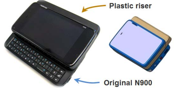
Fig. 3. Spectrum sensor prototype implementation on N900 mobile phone.
