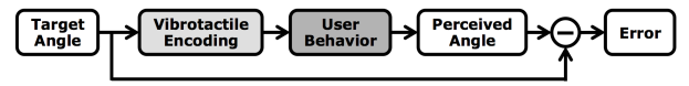
Figure 5: Calculation of the resulting lateral angle deviation, influenced by the vibrotactile encoding due to quantization and user errors due to misinterpretation of patterns.
