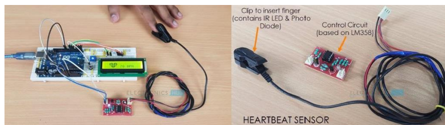
Fig. 4. Heartbeat Sensor Module with Probe (finger based)
