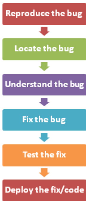
Figure 1. Typical Debugging Process using Traditional Methods
