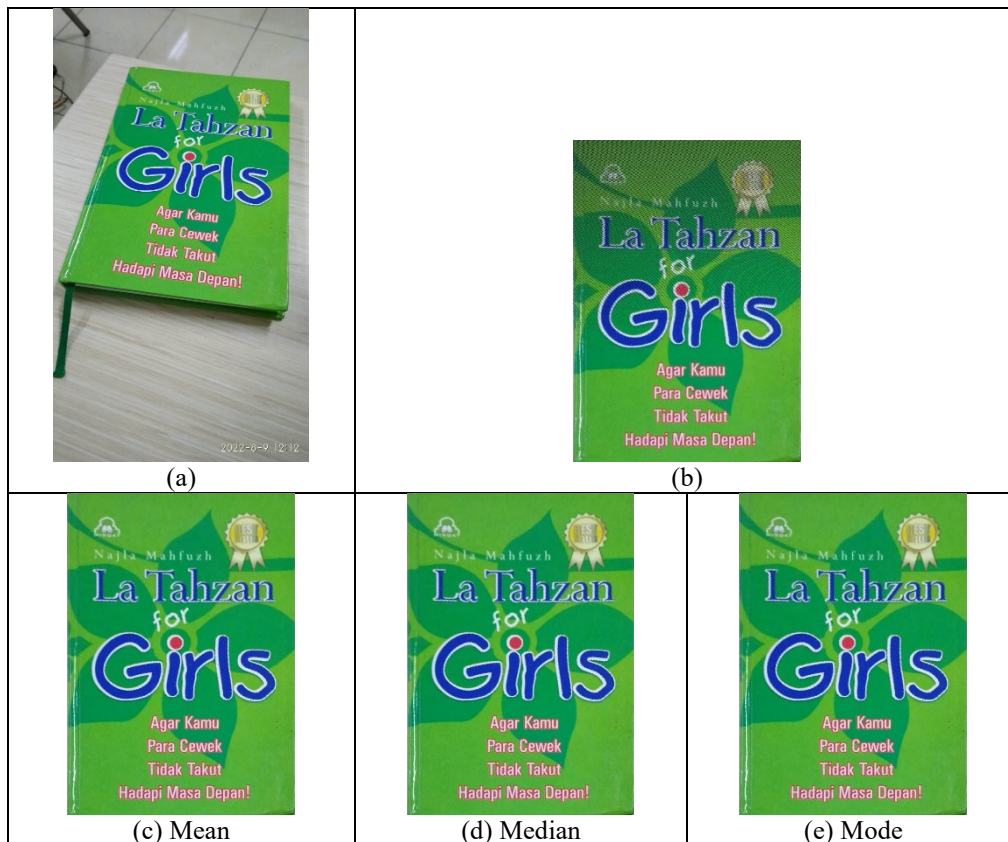
FIGURE 9. (a) picture of the original document from the camera, (b) pictures document after conducted transformation perspective however still perforated, ( c, d, e ) picture document after filling the hole using the mean, median, and mode method.
