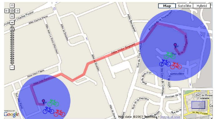
Figure 2: The mobile network moves and crosses different access networks (Wi-Fi, GPRS)
