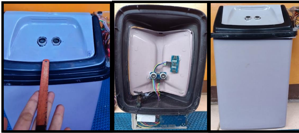
Fig 4. Testing on Object Detecting Sensors, Ultrasonic Sensors and Buzzers
