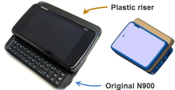
Fig. 3. Spectrum sensor prototype implementation on N900 mobile phone.
