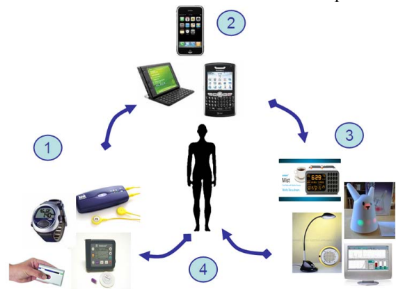
Fig. 1. Sentient components and operation. 1) the user wears a physiological sensor, 2) the algorithm detects an emotional state, 3) the smartphone interacts with the user and the environments, and 4) the user receives feedback.
