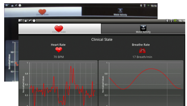
Figure 5. The developed cardiac, respiratory and motor activity graphical interface implemented on the Android OS tablet computer
