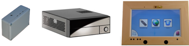
Figure 1. eHome system: multi-sensor-box, central server and local user interface (illustration not to scale)
