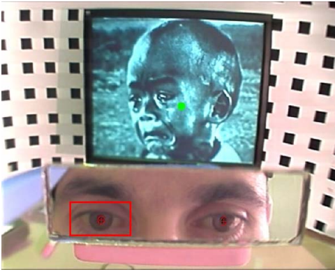
Fig. 3. Example of a single frame captured by the camera. The rectangular area marked by red represents the ROI.
