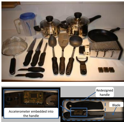
Figure 4. Overview of the sensor embedded kitchen utensils (top); kitchen knife with an embedded wireless accelerometer (bottom).
