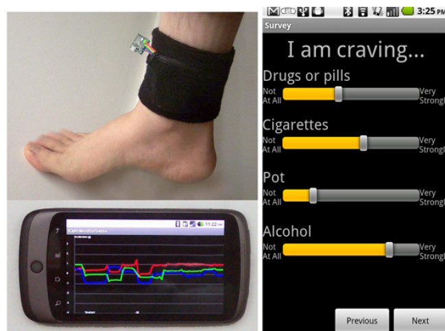
Fig. 1. (top) Photograph of ankle sensor band; (bottom) display of real-time physiology data; and (right) sample EMA screen on mobile phone. Intervention message not shown.
