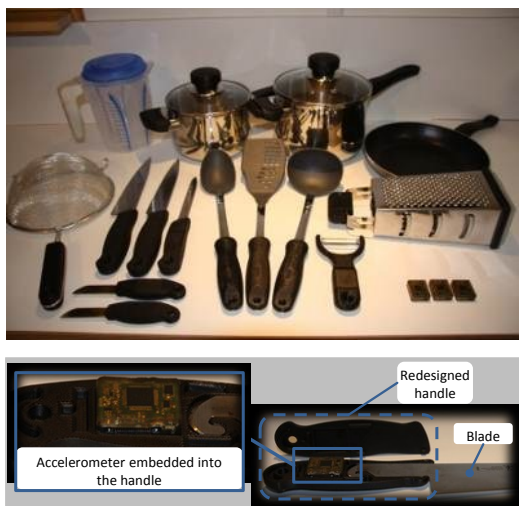
Figure 4. Overview of the sensor embedded kitchen utensils (top); kitchen knife with an embedded wireless accelerometer (bottom).
