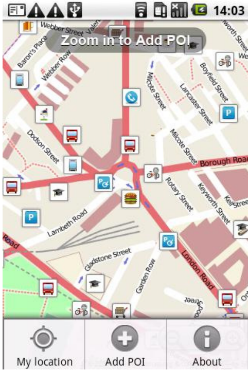
Fig. 5. The Mapzen POI collector for OpenStreetMap. The screenshot shows the application working on an Android mobile phone
