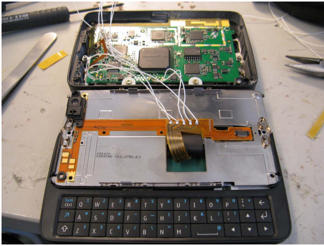
Fig. 1. The spectrum sensor detector board inside N900 mobile phone.
